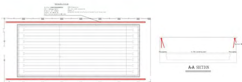
One Durkeesox air duct is installed on the two sidewalls respectively to realize uniform air supply and it's appearance bleed perfectly with the decoration style and to prevent condensation effectively on sidewall glass curtain
